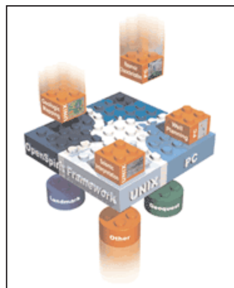
Figure 1: OpenSpirit is a platform-independent, plug-and-play framework that communicates between various vendor databases and applications which haven't been pre-designed for interoperability.
